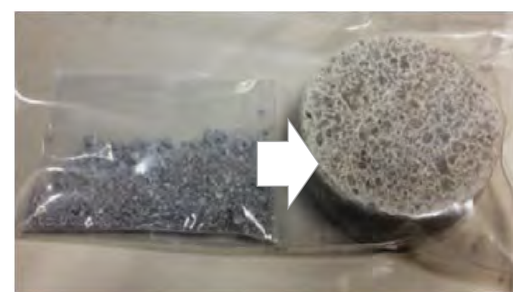
Recycling of crushed concrete
